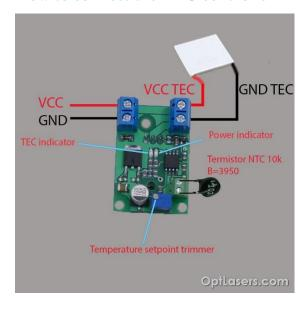
TECs can be connected parallel or in series. Please remember that high current needs proper wiring with bigger cross section of the cables.
