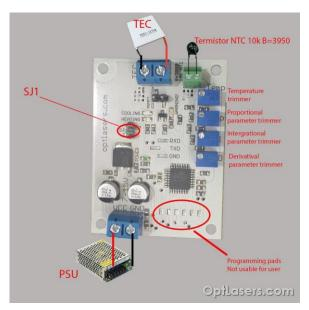
It is possible to connect TEC in two ways. Depending on the chosen connection, different side of the TEC can be cold while cooling:
