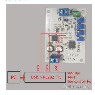
TXD should be connected to RXD
