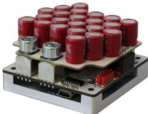
Diode driver is designed to supplying the laser diodes and diode arrays by pulsed current up to 200A or DC current up to 64A. Produced as an OEM module. The driver provides a wide range of smooth change of parameters of radiation.
