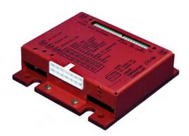
Redwave Linear Temperature Controllers come in three different types: LTC-25, LTC-50 and LTC-100 with maximum current capabilities of 2.5A, 5A and 10A, respectively, single supply operation (+5→30V) and temperature stability down to 0.001K. All models provide a variable current limiter up to the maximum current, various sensor capabilities (thermistors, RTDs, AD590, LM335), variable P-I setting, LED monitors and remote shutdown.
