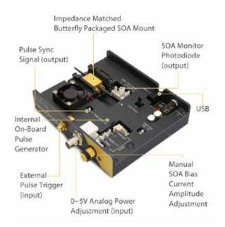
A CW laser diode is used as the input to the SOA. When the bias current driving the SOA is switched ON/OFF in a pulsed mode (with adjustable speed up to > 1 GHz), the result is a fiber optic modulator which offers multiple advantages over traditional modulator technologies. These units can be configured for wavelengths from 750 nm to 1700 nm. It is a lossless, high extinction ratio and highly polarized modulator solution.
