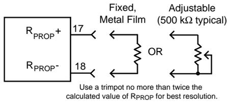
$$R_{PROP} = \frac{500 \text{ k}\Omega}{\text{GAIN}} - 5 \text{ k}\Omega$$
