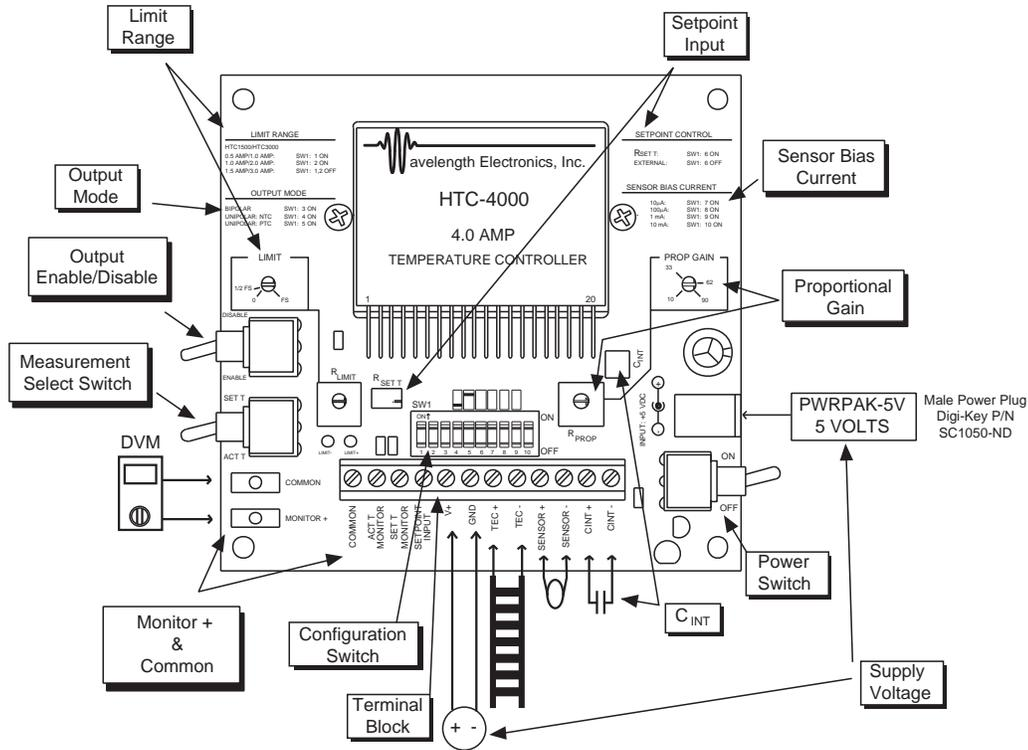
**To Install the HTC on the HTCEVALPCB Evaluation Board with HTC Heatsink**
