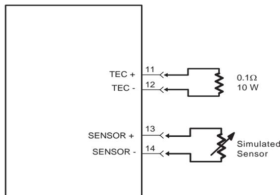
Values shown can simulate any load up to the HTC Series maximum of 4 A.
