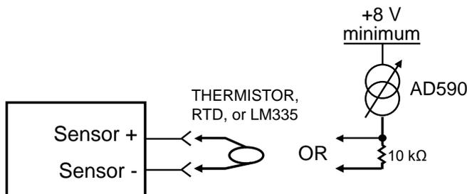
Virtually any type of temperature sensor can be used with the HTC. It must produce a feedback voltage between 0.25 V and (V+ minus 1.3 V). See Step #3 ( $R_{BIAS}$ ) to set the bias current to the sensor.
