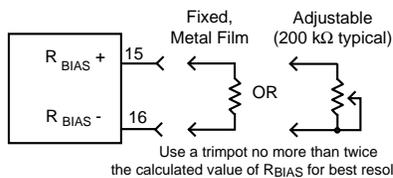
$R_{BIAS}$  determines the bias current sourced to the sensor attached at pins 13 & 14. The chart indicates recommended currents for typical sensors. When using a voltage feedback sensor (such as an AD590), leave pins 15 & 16 open.
