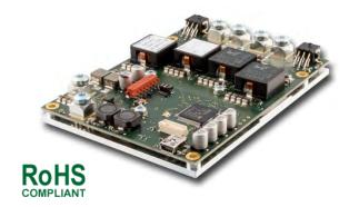
The TEC-1123 is a specialized TEC Controller / power supply able to precision-drive two independent Peltier elements.
