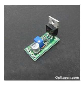
By selecting an appropriate PSU for the driver in question, it is possible to power literally every laser diode available on the market up to 5W - 405 nm, 445 nm, 520 nm, 638 nm, 650 nm, 808 nm, 980 nm. The examples of diodes are: 1 W 445 nm, 3,5 W 445 nm, 6 W 445nm, 700 mW 635 nm, 200 mW 808 nm, 1 W 808 nm, 5 W 808 nm, 1W 520nm.
