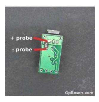
We recommend to check/set the current using a test load resistor because it is much safer and will limit the possibilities of mistake.
