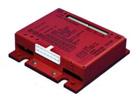
Redwave Linear TEC Temperature Controllers come in three different types: LTC-25, LTC-50 and LTC-100 with maximum current capabilities of 2.5A, 5A and 10A, respectively, single supply operation ( $+5\rightarrow30V$ ) and temperature stability down to 0.001K. All models provide a variable current limiter up to the maximum current, various sensor capabilities (thermistors, RTDs, AD590, LM335), variable P-I setting, LED monitors and remote shutdown.
