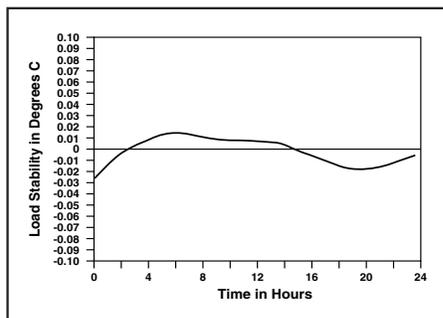
With a typical drift within 0.01 $^{\circ}$ C over a 4 hour period, the LDT-5412 out-performs similar thermoelectric temperature controllers.
