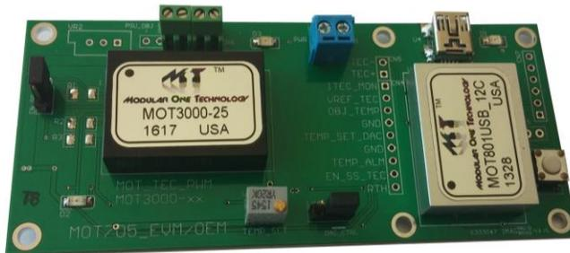
Voltage, and measure the object temperature. The set temperature can be programmed into an integrated EEPROM. This feature allows power cycling whilst maintaining the last programmed temperature setting. The temperature setting DAC is powered through the main board power supply in order to maintain the set temperature when the USB is disconnected.
