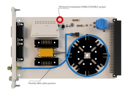
2. Connect jumper to enable the on-board modulation.
