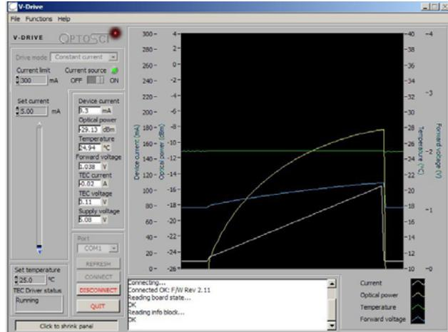
The LDR1000E laser driver module provides a versatile and user friendly platform for stable current and TEC control of laser diodes, SOAs, SLDs, 980nm pump lasers etc. The fully integrated digital Eurocard modules are designed for device characterisation, prototype development and experimental systems and offer easy device integration, full PC control and monitoring, or set & forget operation utilising the on-board EPROM.
