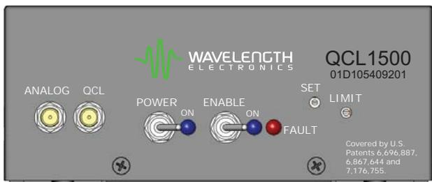
Figure 1. QCL Driver Front Panel
