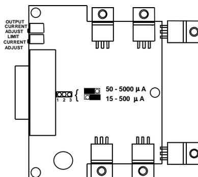
The factory set photodiode range is 50 $\mu$ A - 5000 $\mu$ A. As shown in the diagram above, the jumper is internal to the unit and behind the connector. To change the setting to the more sensitive range (15 $\mu$ A - 500 $\mu$ A), move the jumper to the back two pins.
