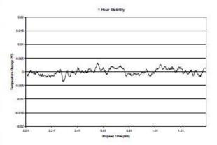
The LDT-5500B demonstrates temperature stability better than ±0.004°C over one hour.
