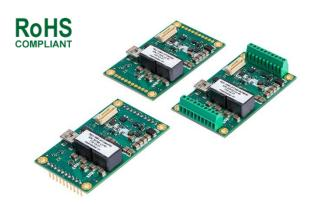
The TEC-1091 is a specialized TEC Controller / power supply able to precision-drive a single Peltier element.
