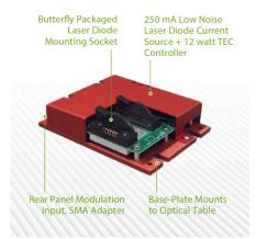
The LD-CONTROLLER-C151 combines a low noise laser diode current source with a high stability TEC controller into a compact, affordable module. The temperature control is fully linear and a separate power supply can be used for the laser TEC if the user wants to optimize for the lowest noise performance. The laser diode current source has an analog modulation bandwidth of 250 kHz. It also offers a separate fast TTL compatible modulation port through an SMA connector.
