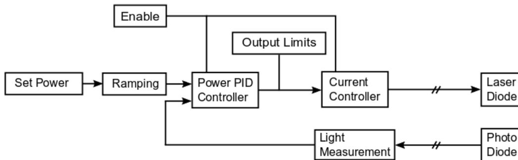
Figure 10. Functional overview of the light power control on LDD-1301/1303.
