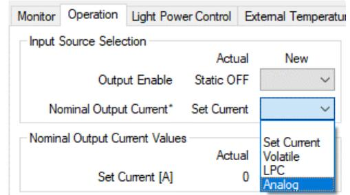
Figure 30. Output Current Setting for Analog Input.
