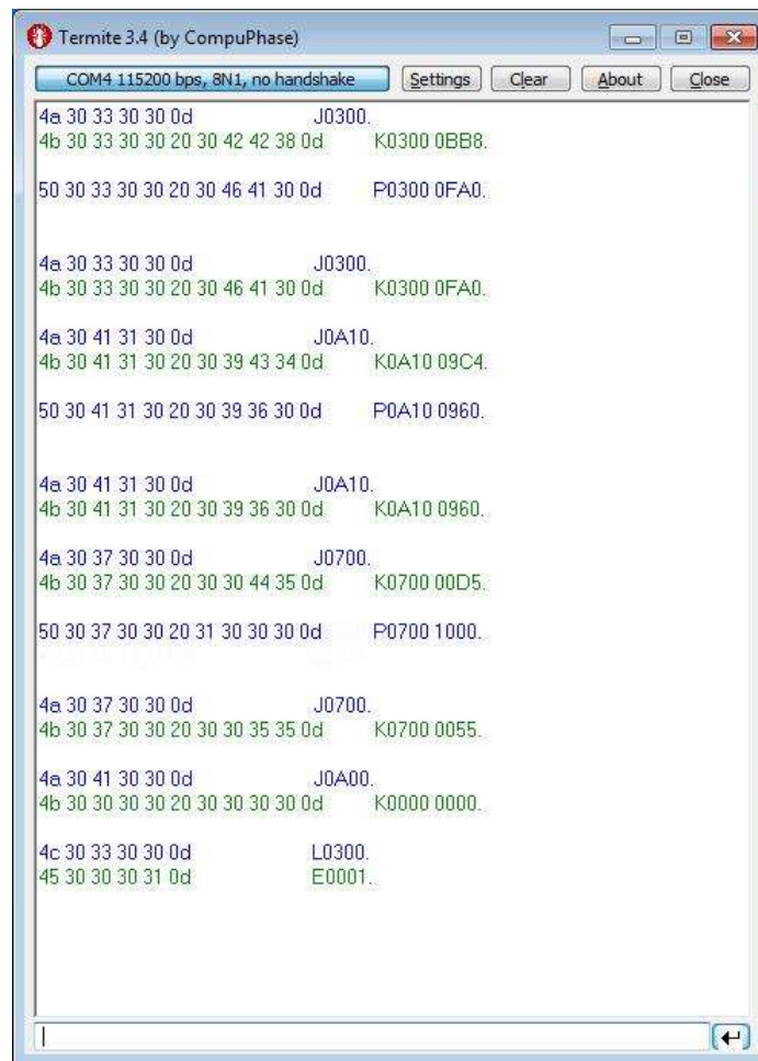
Fig. 10 – Screenshot from the Termite terminal with commands and answers
