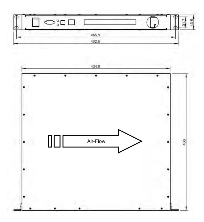
All dimensions are in mm Rack mounting brackets are removable
