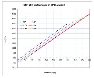
interface quality between the diode and cold plate, and ambient temperature. Users are advised to manually ramp the TEC driving current after assembling the diode on the cold plate to identify the optimum current and set current limit accordingly so that the TEC will not runaway.
