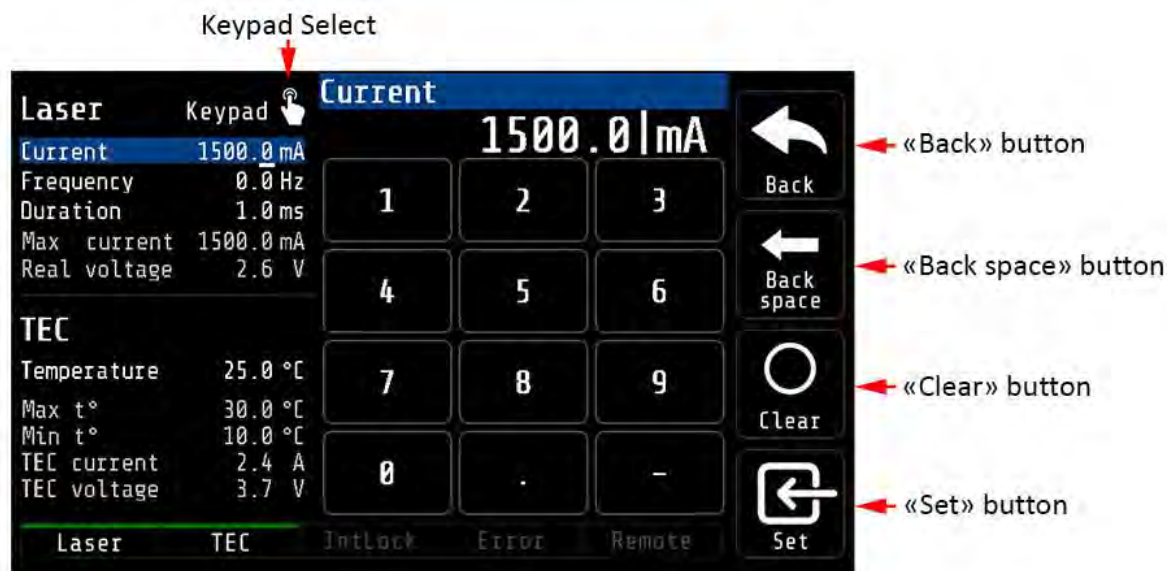
Fig. 14 – The I Current Keypad screen
