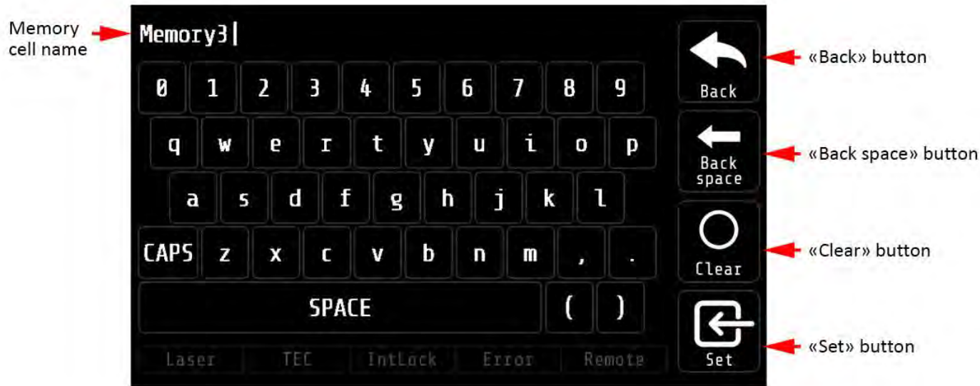
Fig. 20 -The Memory Keypad screen
