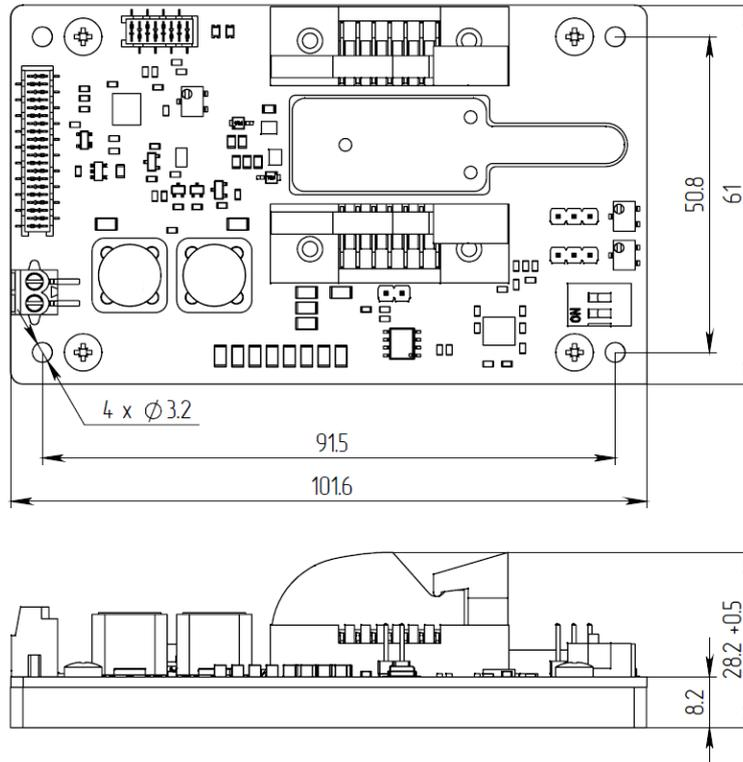
**26.4. SF8xxx-ZIF14 model with Azimuth connectors for 14-pin Butterfly**
