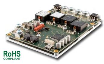
The TEC-1122 is a specialized TEC Controller / power supply able to precision-drive two independent Peltier elements.
