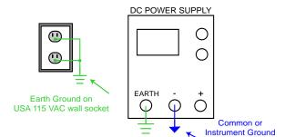
Unless Earth and Instrument Ground are connected via the power supply, Instrument Ground is floating with respect to Earth Ground
