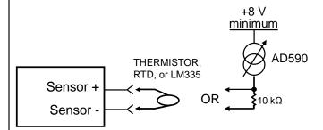
Virtually any type of temperature sensor can be used with the HTC. It must produce a feedback voltage between 0.25 V and (V+ minus 1.3 V). See Step #3 ( $R_{\rm BIAS}$ ) to set the bias current to the sensor.
