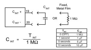
$C_{\rm int}$  sets the integral time constant of the system from 0 to 10 seconds. Use a capacitor with Dissipation Factor less than 1% for best performance. These typically include metallized film polyester, polypropylene & some ceramic capacitors. Capacitors with Dissipation Factors >1% (typically electrolytic, tantalum, and ceramic) will cause drift in the Integrator circuit. To disable the integrator, use a 1 M $\Omega$  resistor across pins 19 & 20.
