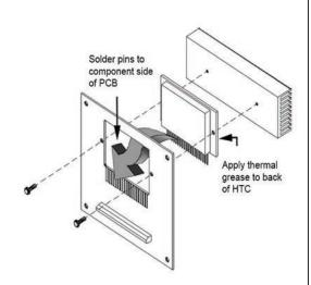
If the HTC is to be used without the HTCEVALPCB board, apply the thermal grease as directed, line up the screw holes in the HTC and heatsink and attach with the supplied screws. Connect the HTC pins to your system by soldering them to the appropriate leads.
