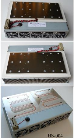
The heatsink we use for OCP-300 is our model HS-004. HS-004 has four heat pipes embedded in the base of the heatsink to minimize heat spreading resistance; the heatsink is nickel plated and the heat pipes are soldered into the heatsink. HS-004 is available for sale as a standalone unit. It is a great solution for high power lasers, electronics, IGBTs, etc.
