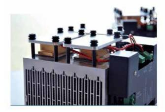
This control and mounting module is used primarily for CW mode. But it is also able to deliver pulses which are generated internally by an on-board pulse generator, or on-demand from an external analog modulation signal. This control and mounting module is very compact and offers an excellent pre-configured solution for OEM integration into your high power laser system.
