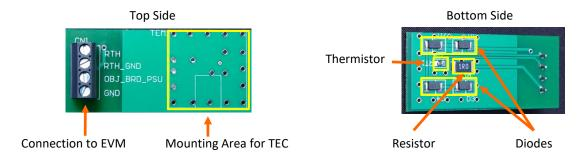
Designed to easily interface to the MOT705\_EVM (see page 4), the current through the diodes and resistor, and hence power dissipation, can be conveniently adjusted via VR2.
