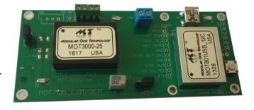
Voltage, and measure the object temperature. The set temperature can be programmed into an integrated EEPROM. This feature allows power cycling whilst maintaining the last programmed temperature setting. The temperature setting DAC is powered through the main board power supply in order to maintain the set temperature when the USB is disconnected.
