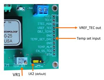
Alternatively the object temperature can be set by an external voltage applied to TEMP\_SET\_DAC on CN4. The reference voltage, VREF\_TEC, is also available on CN4 and can be used as a reference for an external DAC. In this mode LK2 should be altered to the optional position.
