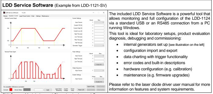
CW Current Modulation and Chopping by Internal Generators.
