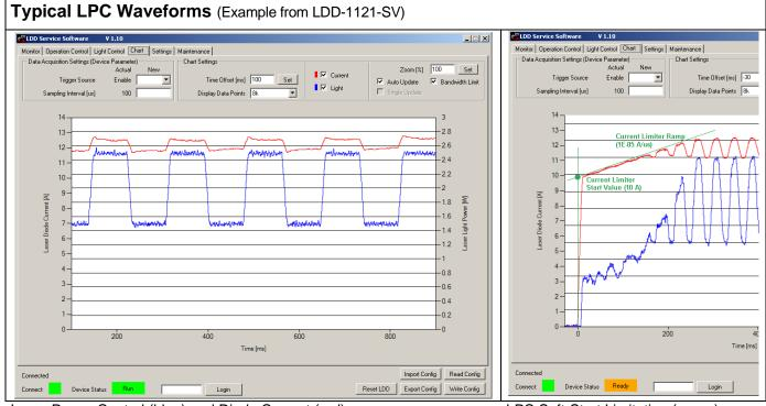
Laser Power Control (blue) and Diode Current (red).
