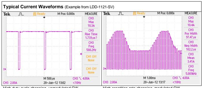
High duty-cycle chopping, unmodulated CW.
