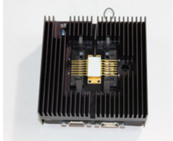
Figure 16. Seat the laser such that the butterfly pins from the butterfly package make physical contact with their corresponding ZIF pins.
