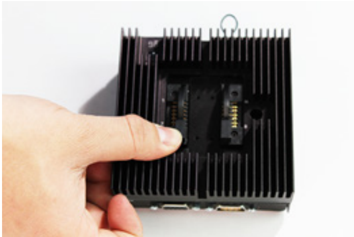
Figure 14. Open the ZIF sockets by pushing on the smaller top clamp, as shown.
