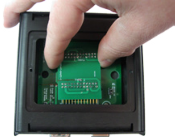
Figure 6. Align the connection card with the 24 pins.
