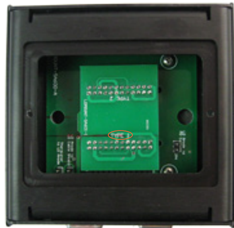
Figure 7. Fully seated, properly installed connection card for a Type 1 laser.
