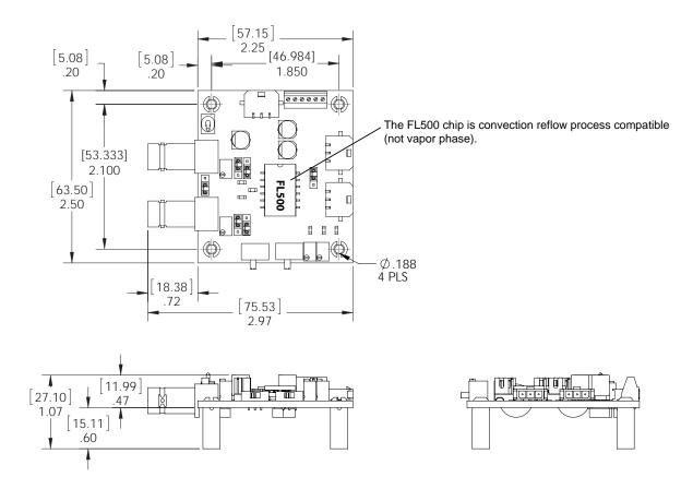
Figure 11. FL591FL Mechanical Dimensions
