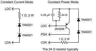
produces approximately 30 mA laser driver current. Vary the resistor value to change the output current.
