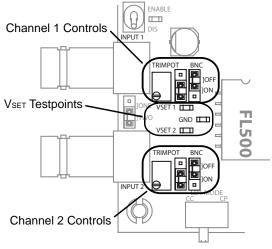
Figure 6. Current Setpoint Section
