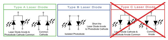
Figure 3. Laser Type Diagrams
