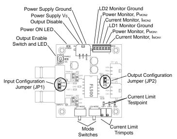
Figure 5. FL591FL Configuration Controls
