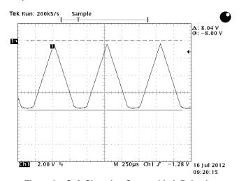
Figure 9. Soft Clamping Current Limit Behavior
