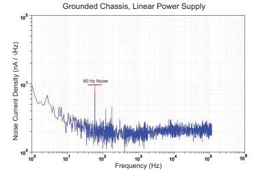
Figure 14. Noise Plot with Grounded Chassis and Linear Power Supplies
