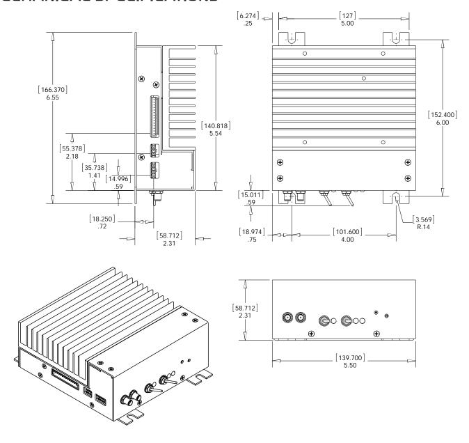
Figure 20. QCL OEM Driver Mechanical Dimensions
