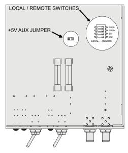
Figure 5. Bottom View of QCL Driver Showing the Internal Remote / Local Switches and +5V AUX Jumper
