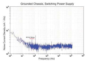
Figure 15. Noise Plot with Grounded Chassis and High Quality Switching Power Supplies
