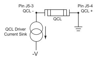
Figure 6. QCL Wiring and Polarity
