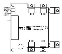
The factory set photodiode range is  $50\mu\text{A}$  -  $5000\mu\text{A}$ . As shown in the diagram above, the jumper is internal to the unit and behind the connector. To change the setting to the more sensitive range ( $15\mu\text{A}$  -  $500\mu\text{A}$ ), move the jumper to the back two pins.
