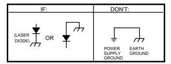
WARNING: If you plan to operate the MPL with an MPT, you may need to use separate power supplies. If the TE cooler or thermistor is connected to the laser diode, you must use two separate power supplies and let each float independent of the other.
