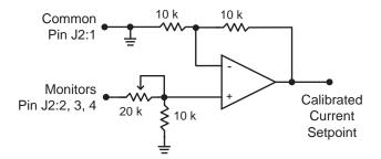
Figure 20. Monitor Calibration Circuit
