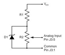
$V_{\text{SV}}$  = Supply voltage (5 to 30 V) D1 = Bandgap reference\* (LM4040) R1 = 2.2 k , 1 W resistor R2 = Trimpot, 10 k to 100 k
