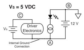
Figure 22. Negative Supply Operation, 5 V Electronics Power Supply
