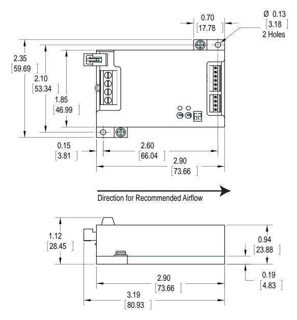
Figure 30. PLDxK-CH Driver Mechanical Dimensions
