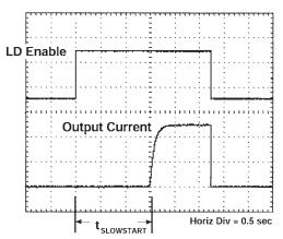
Figure 24. Output Turn-On Delay
