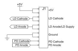
Figure 17. Revision A Connector PLD5K-CH and PLD10K-CH
