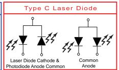
Figure 3. Laser Type Diagrams
