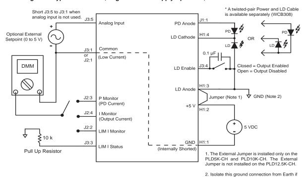
Figure 8. Type A & B Lasers, Negative Power Supply Operation; PLD5K-CH and PLD10K-CH
