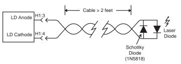
Figure 18. Long Cable Laser Protection
