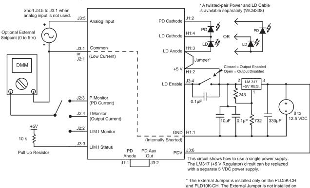
Figure 7. Type C Laser Diode; PLD5K-CH and PLD10K-CH
