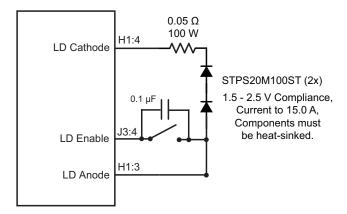
Figure 4. Constant Current Mode Laser Test Loads
