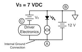
Figure 23. Negative Supply Operation, 7 V Electronics Power Supply
