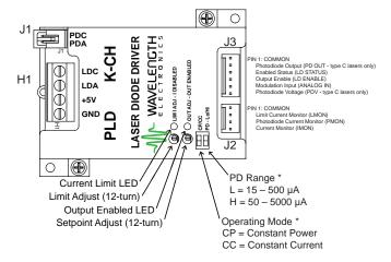
Figure 12. PLD Driver Adjustments and Controls
