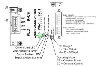
Figure 1. PLDxK-CH Driver Controls
