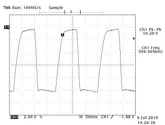
Figure 35. 600 kHz Output Plot QCL1500 at 1.15 A with 10  $\Omega$  Test Load
