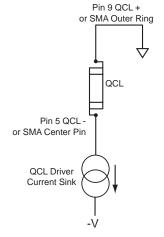
Figure 7. QCL Polarity Diagram
