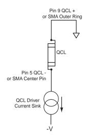
Figure 4. QCL Polarity Diagram
