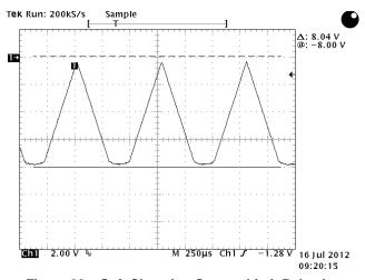
Figure 33. Soft Clamping Current Limit Behavior
