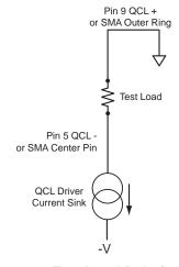
Figure 13. Test Load Polarity Diagram
