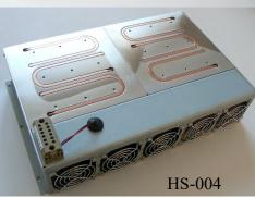
The heatsink we use for OCP-300 is our model HS-004. HS-004 has four heat pipes embedded in the base of the heatsink to minimize heat spreading resistance; the heatsink is nickel plated and the heat pipes are soldered into the heatsink. HS-004 is available for sale as a standalone unit. It is a great solution for high power lasers, electronics, IGBTs, etc.
