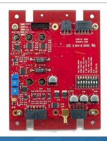
Operating Manual C158 - Laser Diode Controller 250mA Laser Output Current
