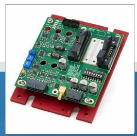
Operating Manual C151 - Laser Diode Controller 250mA, Type-1 Pin Configuration
