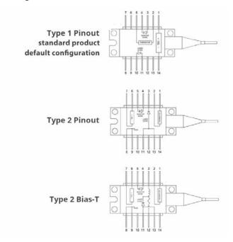
The standard model is for a type 1 pin configuration.
