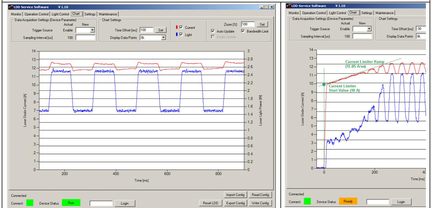
Laser Power Control (blue) and Diode Current (red).
