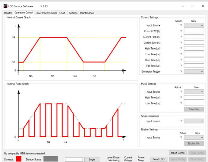
The included LDD Service Software is a powerful tool that allows monitoring and full configuration of the LDD-1124 via a standard USB or an RS485 connection from a PC running Windows.
