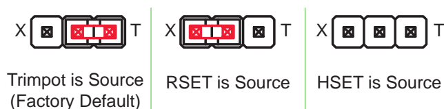
Figure 7. VSET Source Jumper Settings
