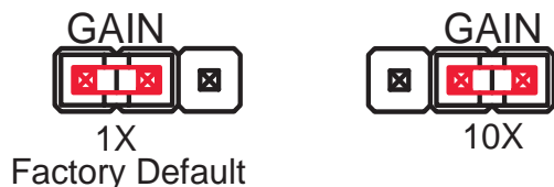
Figure 9. Sensor Gain Jumper Settings
