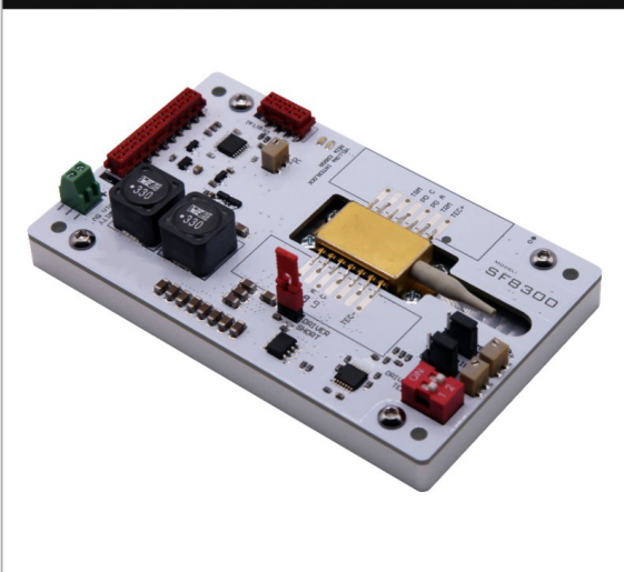
LASER DIODE CONTROL ELECTRONICS & MOUNTING MODULE
